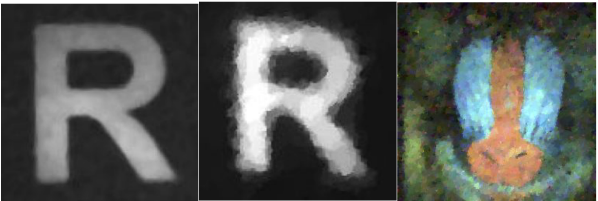
Sample image reconstructions from single-pixel camera. (a) 256 \times 256 conventional image of a black-and-white “R”. (b) Image reconstructed from M = 1300 single-pixel camera measurements ( 50 \times sub-Nyquist). (c) 256 \times 256 pixel color reconstruction of a printout of the Mandrill test image imaged in a low-light setting using a single photomultiplier tube sensor, RGB color filters, and M = 6500 random measurements.
